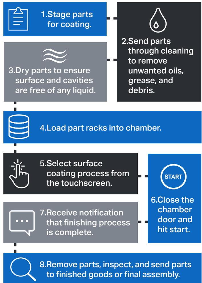
a metal ceramic that is two- to three-times harder than plated chrome – providing the desired look and a longer lasting finish. The ability to create chrome finishes without plating chemistries offers opportunities for manufacturers to deliver chrome coatings while committing to an environmentally sustainable process.
