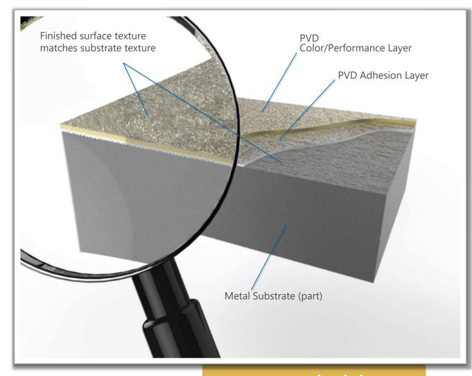
...vaporize it in a vacuum, and deposit it, atom-by-atom, onto a surface.
